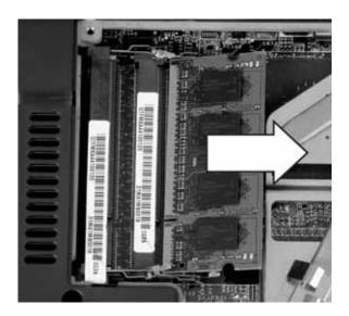
12 Hold the new or replacement module at a 30-degree angle and press it into the empty memory slot. This module is keyed so it can only be inserted in one direction. If the module does not fit, make sure that the notch in the module lines up with the tab in the memory bay.
