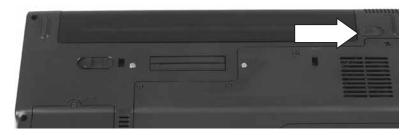
Slide the battery release latch, then slide the battery out of the notebook.
