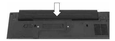
**4** Slide the battery lock to the locked position.
