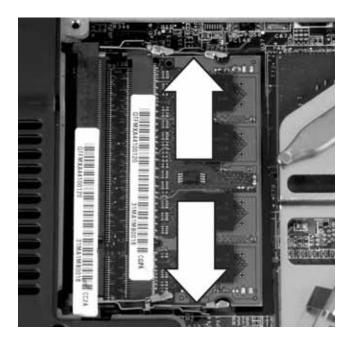
11 Pull the memory module out of the slot.
