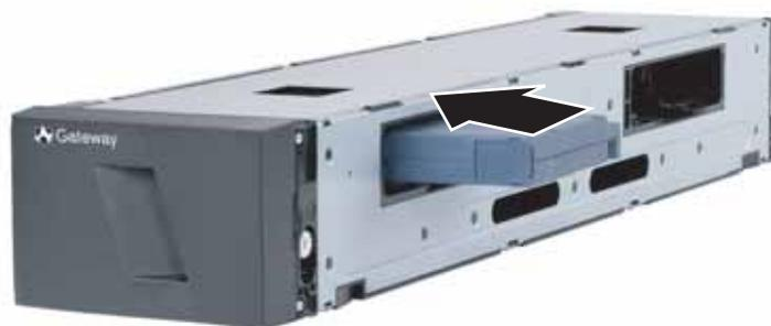
When pushing the cartridge into the slot, you should feel a small resistance (detente) until the cartridge is correctly latched into the slot. All forward progress stops when the cartridge is fully inserted.
