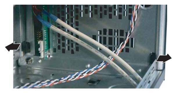
**3** Position the computer where you can grasp the front bottom edge of the bezel, then pull the bezel out and away from the case.
