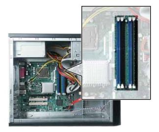
**3** If you are removing a DIMM from the memory module bank, gently pull the plastic tabs away from the sides of the memory module and remove it.
