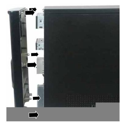
**2** Press the bezel firmly into place.
