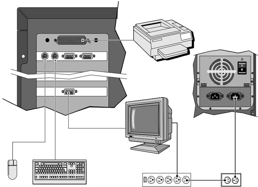
*Figure 1: Connecting Peripherals*
