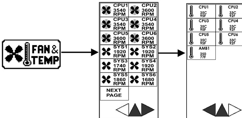
Figure 11: Fan and Temperature Menu
