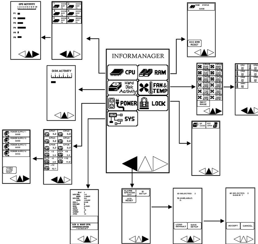
Figure 7: Diagram of LCD Menus
