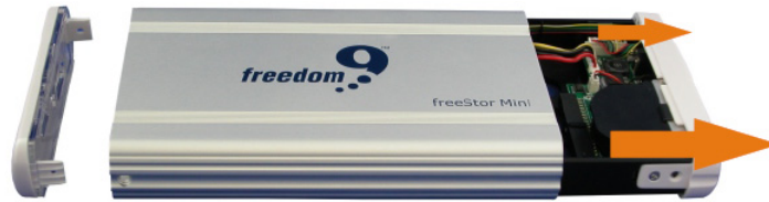
Figure 7: Removing the Tray
