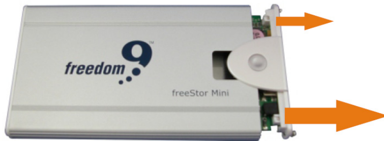
Figure 2: Removing the Connector
