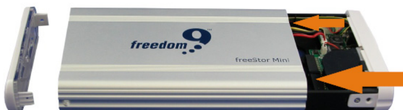
Figure 11: Inserting the Tray
