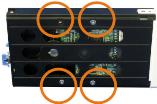
Figure 9: Attaching the Hard Drive Screws
