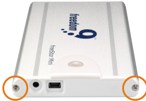
Figure 1: Screws to Remove
