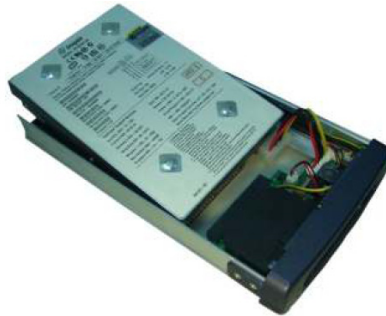
Figure 8: Inserting the Hard Drive
