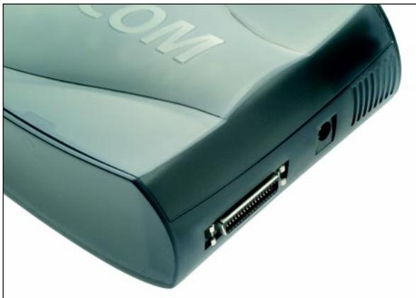
***Note: do not cover the ventilation holes; these are essential for maintaining the correct operating temperature for the FHD-1.***
