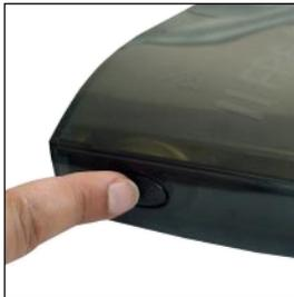
The FHD-1 is equipped with a SYNC button which enables you to synchronize files between your workstation and the FHD-1 (and vice versa).
