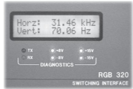
Figure 3-10. Six Diagnostic LEDs on the Front Panel
