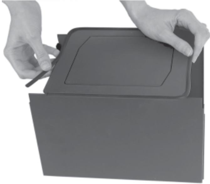
Figure B-3 — Installing protective strips
