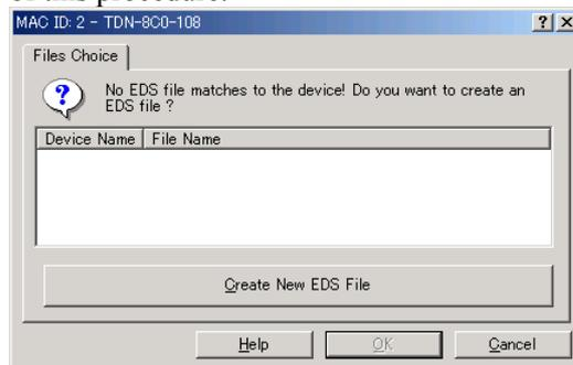
To create a new EDS file based on the data from the device, click the **Create New EDS File** button.
