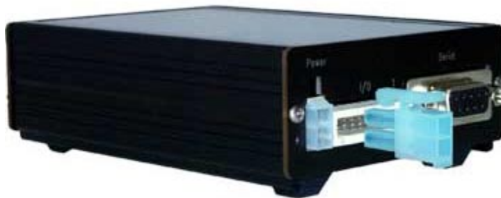
Figure 4: Connecting The Power Supply To Spider SA
