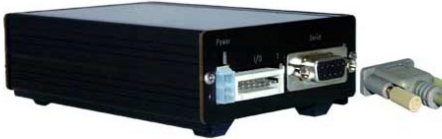
Figure 5: Connecting the Serial Cable to Spider SA
