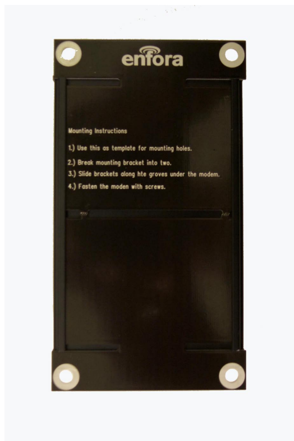
Figure 15: GSM/GPRS Spider SA Mounting Bracket (ready to mount)
