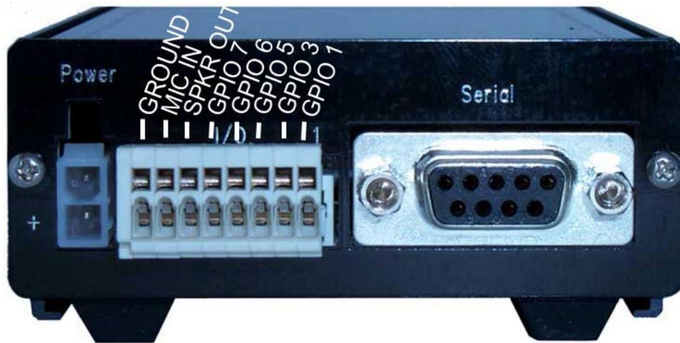
Figure 11: GPIO Pin Configuration
