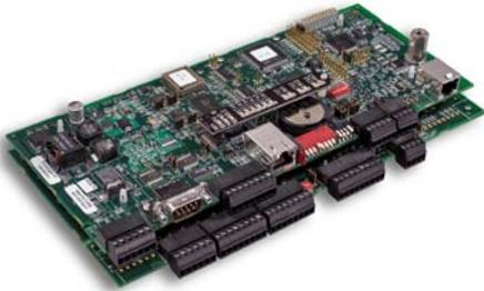
The I/O module (bottom card) provides a mix of analog and digital inputs and outputs that are a perfect fit for small RTU applications.
