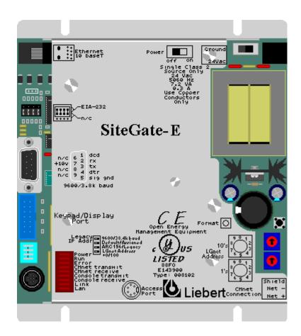
**DESCRIPTION:** The SiteGate-E provides communications between a SiteScan workstation and a control module network (ARC156) consisting of up to 32 control modules. The SiteGate-E provides one Ethernet Console Port and one serial port for direct connection. The Ethernet port is designated meets the IEEE 802.3 standard. The serial console ports are switch selectable for baud rates up to 38.4k bps. Communication between the SiteGate-E and the ARC156 network is provided through an EIA-485 port.
