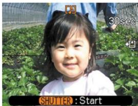
4. Press the shutter button to start audio recording.
