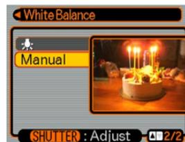
4. Point the camera at a white paper or similar object under the lighting conditions for which you want to set the white balance, and then press the shutter button.
