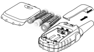
Each radio requires three AAA batteries (not supplied) for power. Batteries are available at your local RadioShack store or online at [www.radioshack.com](http://www.radioshack.com). You can also use Ni-Cd/Ni-MH rechargeable batteries in the radio and recharge them using an optional 6V, series regulated, 1A AC/DC adapter, available at your local RadioShack store. It takes 6 hours for Ni-CD and 12 hours for Ni-MH batteries to charge.
