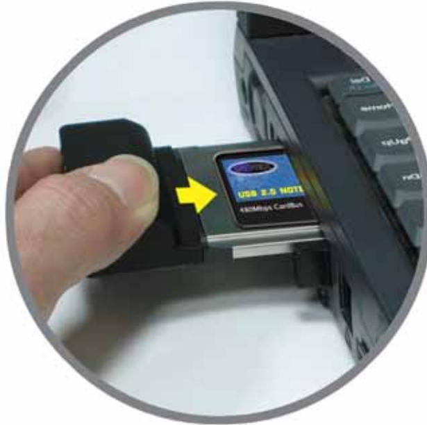
3. When the card bus adapter is inserted into the slot completely, Windows will detect the host controller automatically.
