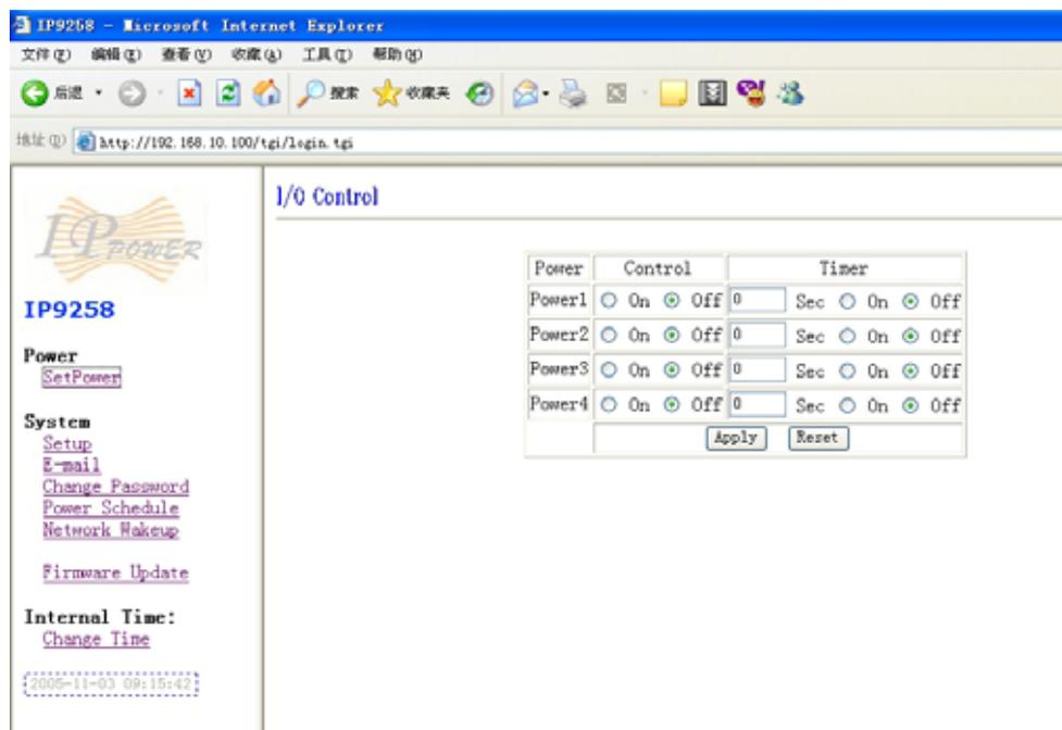
IP Power 9258 can control 4 outputs individually at the same time. User can choose power on or power off with an electrical outlet. User may fill in the corresponding columns with the delay time you wish in seconds, then choose the action after delay to be **on** or **off**.
