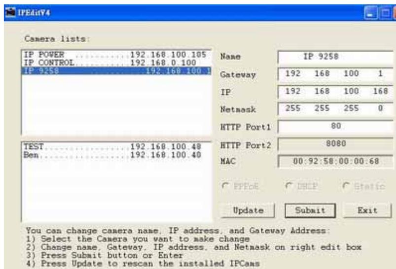
3. Click the equipment's name that you want to edit in the left of the window; it will turn fuscous, the equipment's name and IP address will display in the windows, you can rename (use numbers and letters). After that, click the update button and the new setting will be work in 20 seconds.
