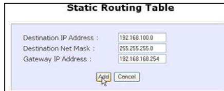
The screenshot shows a window titled "Static Routing Table". It contains three input fields: "Destination IP Address" with value 192.168.100.0, "Destination Net Mask" with value 255.255.255.0, and "Gateway IP Address" with value 192.168.168.254. Below the fields are two buttons: "Add" and "Cancel". A mouse cursor is pointing at the "Add" button.
