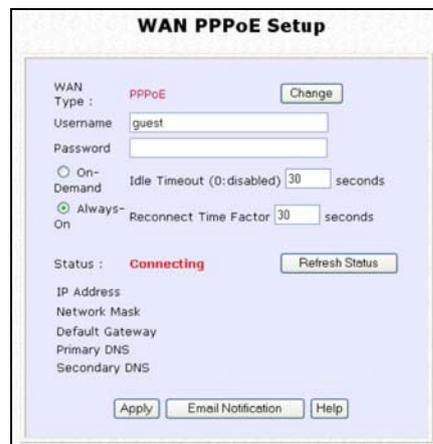
The **Idle Timeout** setting is associated with the **On-Demand** option, allowing you to specify the value (in seconds) after which the access point will disconnect from the ISP after the last Internet activity. A value of "0" will disable idle timeout. **Reconnect Time Factor** is associated with the **Always-on** option and specifies the maximum time the access point will wait before re-attempting to connect with your ISP. Hit the **Apply** button and **Reboot** the access point.
