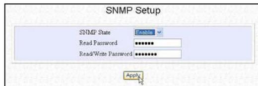
The screenshot shows a window titled "SNMP Setup". Inside the window, there are three fields: "SNMP State" with a dropdown menu showing "Enable", "Read Password" with a text input field containing "public", and "Read/Write Password" with a text input field containing "private". Below these fields is an "Apply" button.
