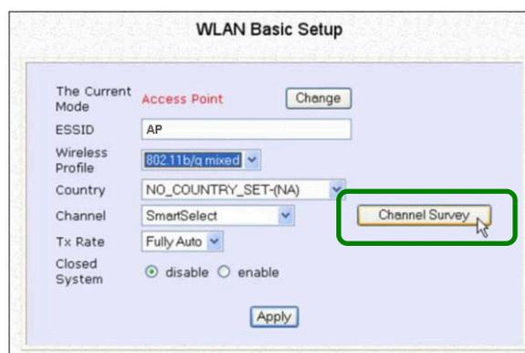
The **Channel Survey** provides a list of the **Freq** (frequency) and **Channel** of the access point detected, the **APCount**, **MyQuality** (your access point's interference from your access point's channel signal) received and **NeighQuality** (interference from the neighbouring access points' channel signals) received.
