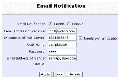
The screenshot shows the 'Email Notification' configuration page. The 'Email Notification' checkbox is checked and labeled 'Enable'. The 'Email address of Receiver' is 'mail@yahoo.com'. The 'IP address of Mail Server' is '192.168.88.43' with the 'Needs Authentication' checkbox checked. The 'User Name' is 'sampleUser'. The 'Password' field is masked with dots. The 'Email address of Sender' is 'send@yahoo.com'. At the bottom, there are buttons for 'Apply', 'Back', and 'Refresh'.
