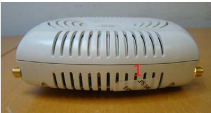
Figure 5 - AP-92 Tel placement front view
