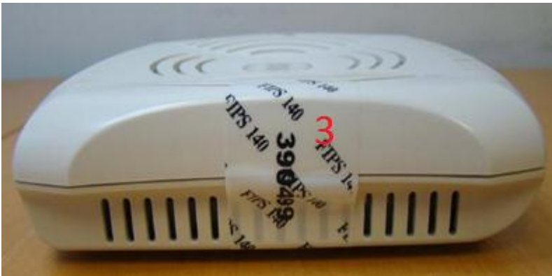
Figure 12 - Aruba AP-93 Tel placement right view
