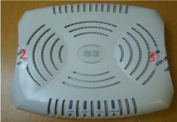
Figure 14 - Aruba AP-93 Tel placement top view
