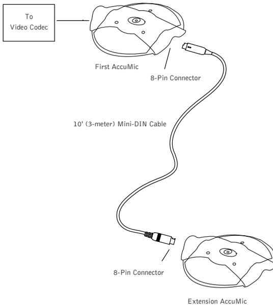
Figure 16. Connecting an AccuMic VC Extension Mic
