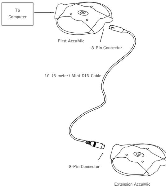
Figure 7. Connecting an AccuMic PC Extension Mic
