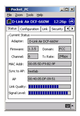
**Link Quality** – Monitors the quality of the data transmission between the Wireless Compact Flash adapter and the Access point
