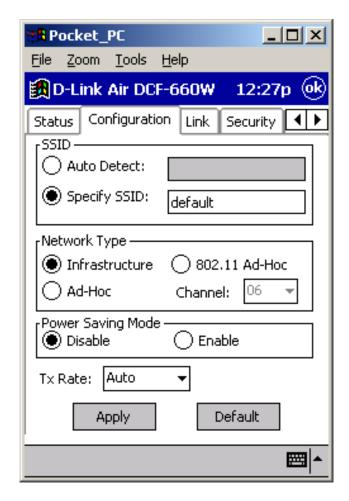
**Power Save Mode –** The Power Save mode is used to extend battery life.
