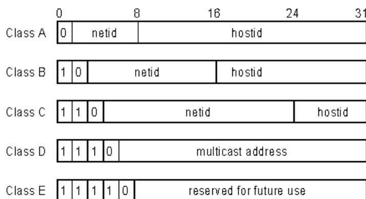
Networks attached to the Internet are assigned class types that determine the maximum number of possible hosts per network. The previous figure illustrates how the net and host portions of the IP address differ among the three classes. Class A is assigned to networks that have more than 65,535 hosts; Class B is for networks that have 256 to 65534 hosts; Class C is for networks with less than 256 hosts.
