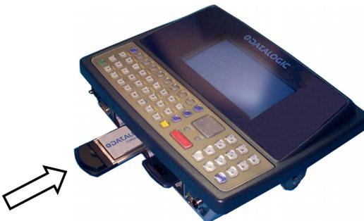
Figure 2 - DOS Terminal Card Installation
