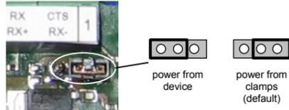
Figure 5–Power Source Jumper Settings
