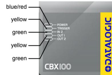
Figure 11 – Indicator LEDs
