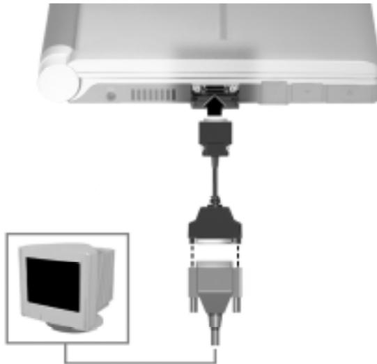
4. Connect the monitor cable to the transfer cable.
