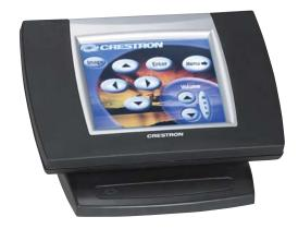
Quick-Touch Pushbuttons—The STX-1700CXP includes a button bezel kit which may be installed to provide ten tactile pushbuttons for quick-touch access to frequently used commands. In standby, the pushbuttons may be operated without waking the touchscreen for extended battery life. Custom engraving of the pushbuttons may be attained using Crestron Engraver software.
