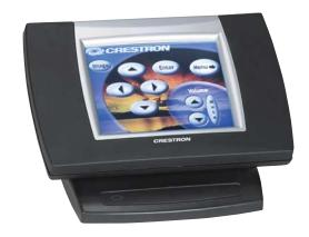
station (included) for easy recharging, simultaneously providing operating power to the touchpanel. The docking station may also be used to recharge a spare ST-BTPN battery pack (sold separately). And if necessary, the touchpanel may even be powered directly using the PW-1215 power pack (included).
