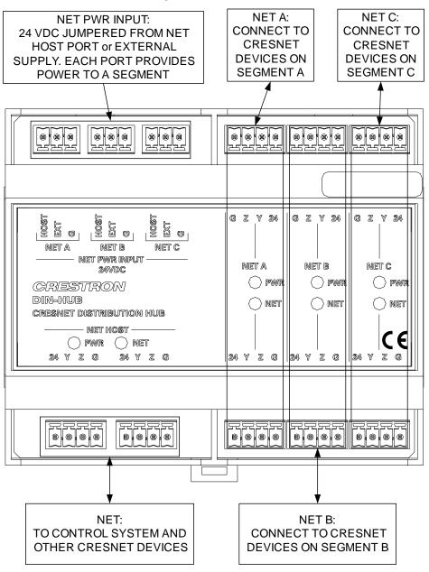
Power can be supplied from a DIN-PWS50 DIN Rail Power Supply or other Cresnet power supply connected to the **NET HOST** port. For more information, refer to the latest version of the DIN-PWS50 Operations & Installation Guide (Doc. 6667), which is available for download from the Crestron website (<a href="www.crestron.com/manuals">www.crestron.com/manuals</a>).
