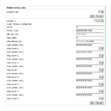
Several options are available in this form. The first, and easiest to understand and use, is the Default Priority value. Output traffic generated by adapters with higher default priority will have preference in the network. The rest of the parameters let you configure two Class of Service criteria (**Criterion I** and **Criterion 2** checkboxes).
