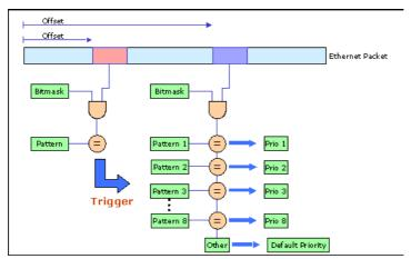
There is one offset, and one bitmask and pattern for the trigger condition. The trigger condition is used to make sure that the Ethernet frame contains, for example, an IP frame. To check this condition, the offset must be set to 16 and the bitmask to 0xFFFF. If the resulting pattern is 0x0800, then the Ethernet frame contains an IP packet and the classification can be made to a known field.
