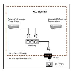
• When you want to isolate the electrical noise produced by some household appliance, because this noise falls in the PLC band and disrupts the signal from the adapters. This setup is illustrated in the picture below.
