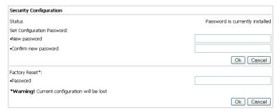
Factory reset will restore the adapter's default settings. The system will ask for the password, which is "betera". Then click **OK**. The adapter will restart with the following configuration:
