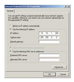
Click **OK** in the TCP/IP Properties window to complete the PC configuration, and click **Close** or the **OK** button to close the Network window.
