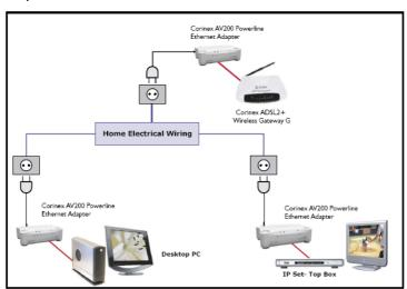
The adapter connected to the ADSL adapter is the access point. Data and video are delivered through ADSL. The access point must prioritize the video higher than other data, to avoid a jittery image whenever there is a heavy data download.
