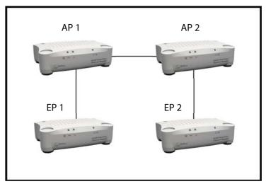
In multi-network scenarios, such as the one depicted in the picture above, there is a new entity, called the QoS controller. The QoS controller's role is to assign channel access to the different networks. The QoS controller acts at the same time as the AP of one of the networks. In the presence of several networks, the coexistence protocol automatically selects one of the APs as the QoS controller.
