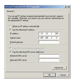
6. Click the **OK** button in the TCP/IP Properties window to complete the PC configuration, and click **Close** or **OK** to close the Network window.
