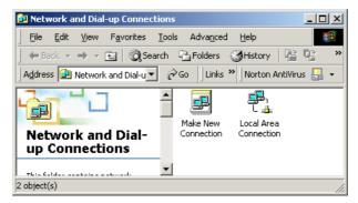
Select the Network and Dial-up Connections icon for the applicable Ethernet adapter (usually it is the first Local Area Connection listed). Do not choose a TCP/IP entry which name mentions DUN, PPPoE, VPN, or AOL. Double click the Local Area Connection. The following window will appear.
