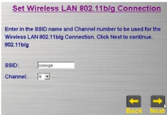
\* Note: the default SSID(ESSID) is "corega", and default channel is 6.
