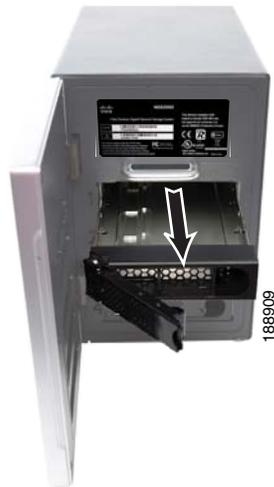
**STEP 6** Position the disk drive into a disk tray. Then, attach the disk drive to the tray by inserting the disk drive screws into the four holes at the bottom of the tray and tightening them with a Phillips screwdriver.
