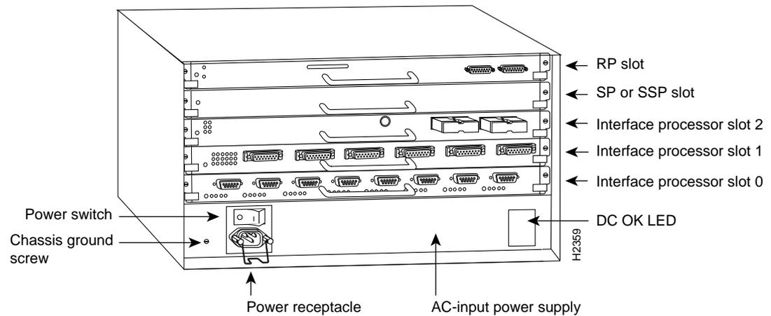
The Cisco 7505 is a five-slot model that provides four interface processor slots. Figure 2 shows the interface processor end of the Cisco 7505. The Route Switch Processor (RSP1), which is a required system component in the Cisco 7505 router, occupies the top slot. The remaining four slots support any combination of interface types: Ethernet, Token Ring, FDDI, and so forth.
