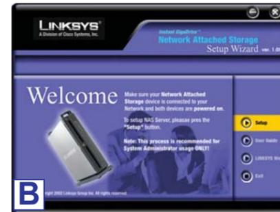
This *Welcome* screen provides you with four options buttons along the right side of the screen. The first button is the **Setup** button. Click this button to continue with the setup procedure. The second button is the **User Guide** button. The third button, **Linksys**, connects you to the Linksys web site if you have an active Internet connection. Lastly, clicking the **Exit** button will exit the Setup Wizard.
