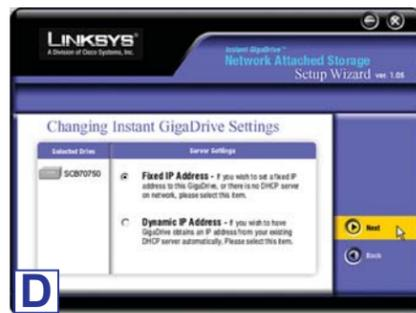
The **Fixed IP Address** is set by default (192.168.1.77). Use this setting if there is no DHCP server on your network and you want the EFG120 to use a static IP Address. With the Fixed IP Address setting, you can also use the EFG120 as your network's DHCP server. Use the **Dynamic IP Address** setting if you already have a DHCP server setting IP Addresses on your network devices.
