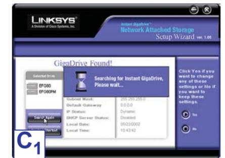
From the screen shown below, once you have found the EFG120 you wish to set up, highlight and click it. Then, click the **Yes** button on the right to change any of the EFG120's settings or the **No** button to accept the settings and exit the Setup Wizard.
