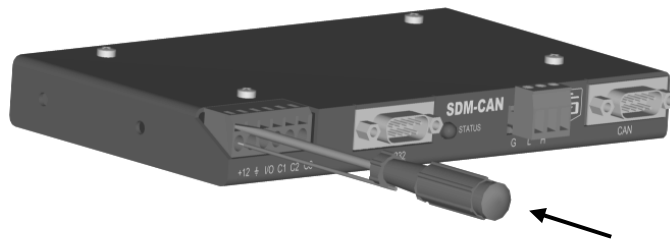
Figure 2-5 Using the Spring Loaded Terminal Blocks (Front Option)
