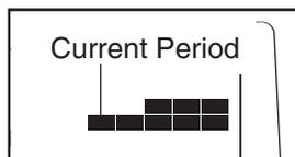
When only three seconds remain in the first period of the program, both the Current Period column and the column to the right will flash and a series of tones will sound. If the speed and/or incline of the treadmill is about to change, the speed setting and/or the incline setting will flash in the display to alert you.
