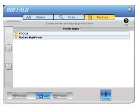
Click the *Profiles* tab to open this page. Use this page to access your profiles. Profiles allow you to save the information associated with a specific wireless network so you can quickly and easily connect to that network when you are in that location. The Profiles page allows you to add, delete, and edit your profiles, as well as import and export data.
