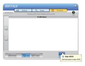
AOSS (AirStation One-Touch Secure System) is a simple, one-touch setup for connecting wireless clients to an access point while enforcing the most secure possible connection encryption type. Users no longer need to worry about choosing the proper security protocols, IP addresses, or SSID. AOSS determines the optimal connection and configures itself in seconds. If your router doesn't support AOSS, turn to page 6 to configure your connection manually with Client Manager or Wireless Zero Config.
