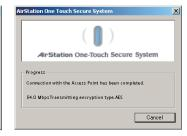
Once AOSS is complete (about 30 seconds), the connection is archived as a profile for later use. To minimize Client Manager to the system tray, click the 'X' in the top right corner.
