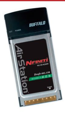
The WLI-CB-AG300NH has three internal diversity antennas. External antennas cannot be attached to the WLI-CB-AG300NH.
