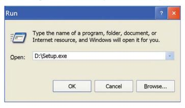
Insert the AirNavigator CD into the CD-ROM drive of the PC. The Air Navigator Setup Wizard launches automatically. If the Air Navigator Setup Wizard does not launch automatically, launch the wizard manually by selecting Start>>Run to open the Run dialog box. Enter D:\Setup.exe in the Open field. D: represents the letter assigned to the CD-ROM drive. If another letter is assigned to the CD-ROM drive, your command should refelect that difference Click the **OK** button to launch the wizard
