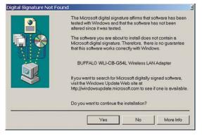
Not Found page opens, informing that no digital signature exists for the driver you are installing, click the Yes button to continue the installation process. When the Wireless Desktop PCI Adapter is successfully installed, click the Finish button. Restart your computer if prompted.
