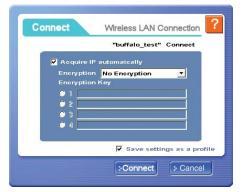
The 'Acquire IP automatically' checkbox tells the client device to obtain an IP automatically from a DHCP server. This is the recommended setting.
