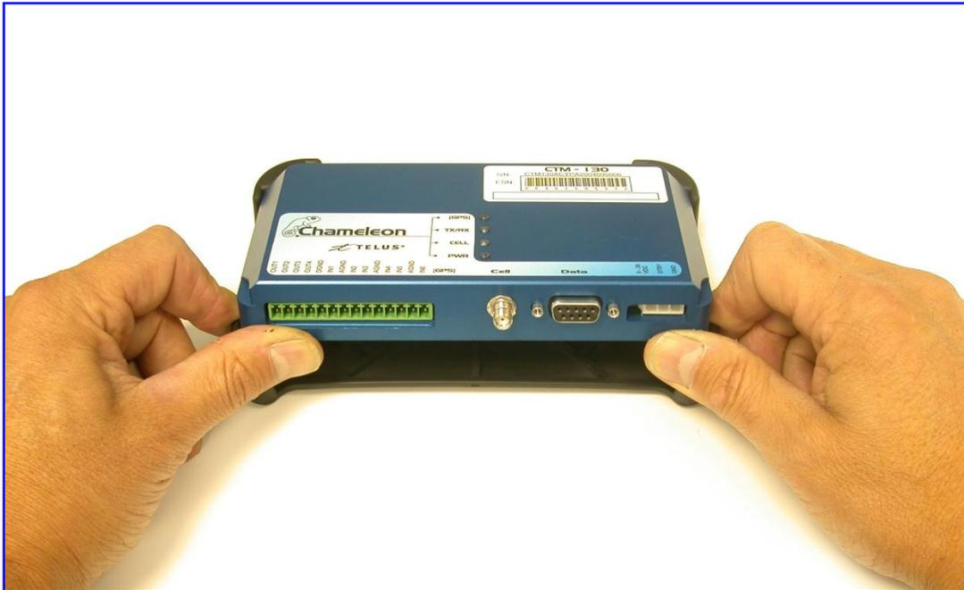
Installing the modem in its base.
