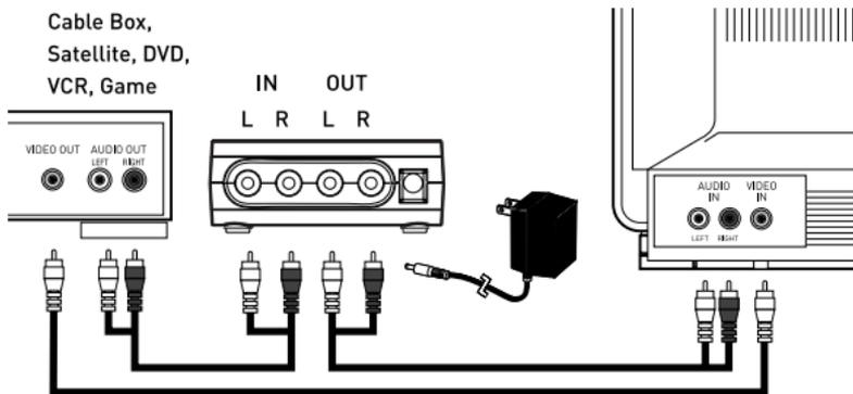
Note: When using RCA cables as shown above make sure that you remove the coax cable from your TV.
