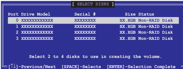
5. Use the up/down arrow key to highlight a drive, then press <Space> to select. A small triangle marks the selected drive. Press <Enter> after completing your selection.
