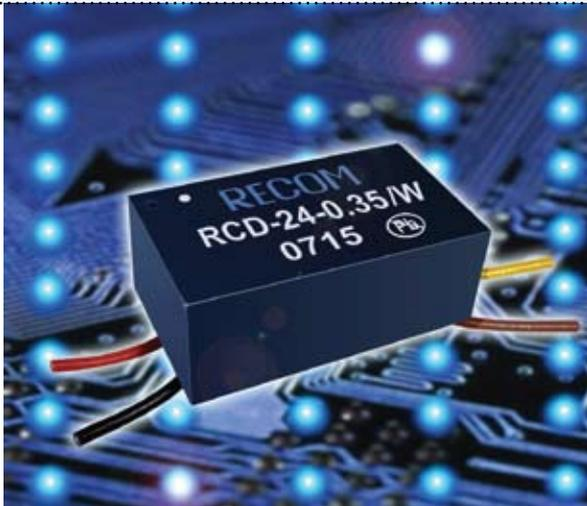
**A new series of integrated, high-efficiency and compact power LED drivers from Recom International will significantly simplify the implementation of LED-based lighting applications.**
