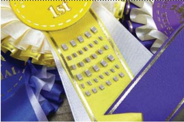
Some Syfer high voltage multilayer ceramic capacitors now offer double the capacitance thanks to breakthroughs in ceramic materials and manufacturing technology. The ability to reduce package size, or increase capacitance range in the same package size, will prove critical to meet today's tight design constraints.
