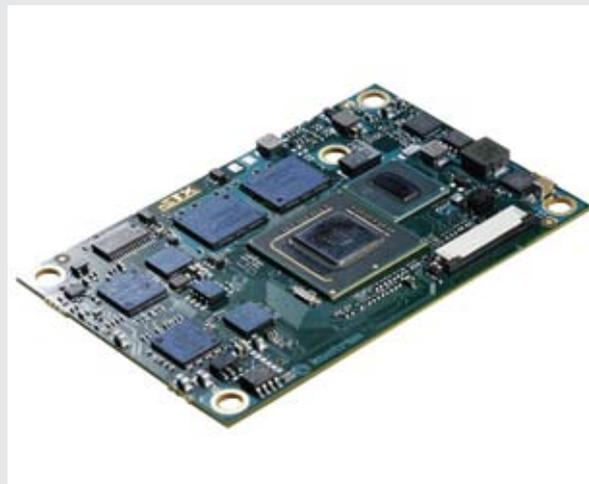
Figure 3: Nano Size Computer On Module from Kontron
