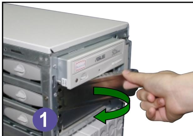
2. From the side of the drive bay, unlock and remove the screwless drive bay lock by turning the knob 45° counter-clockwise until it clicks on the reference point near the “unlocked icon.”
