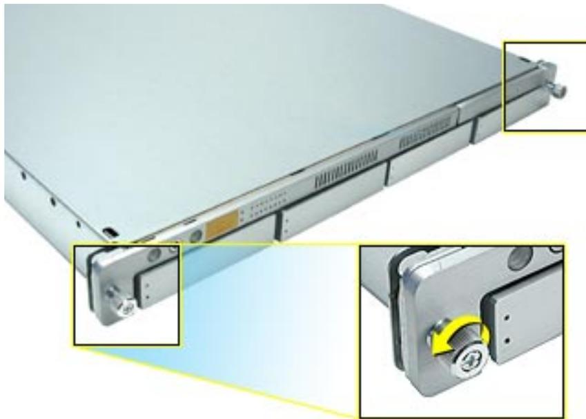
8. Grasp the thumbscrews and slide the bottom housing forward part way to expose the two chassis levers. **(Figure 2)**
