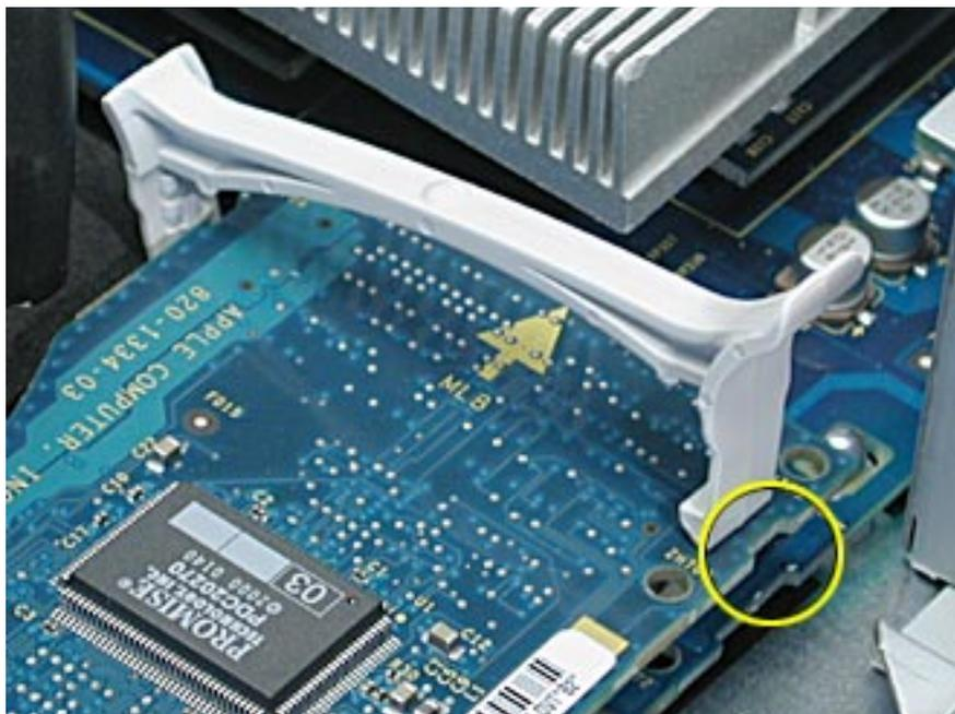
9. Replace the heatsink duct on the heatsink.
