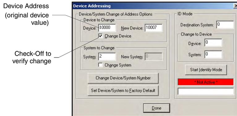
FIG. 25 Device Addressing dialog (changing the device value)
