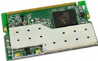
FIG. 1 NXA-PCI80211G mini-PCI Wireless Card
