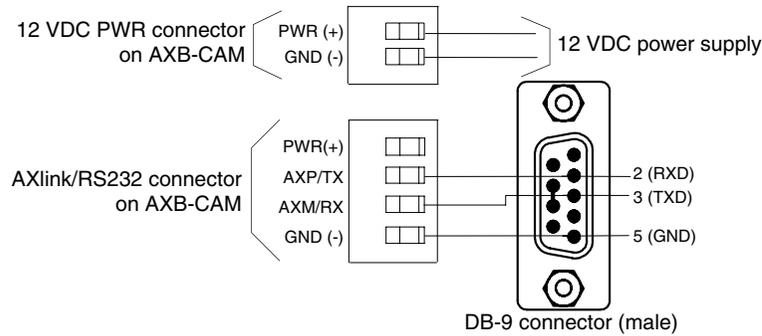
FIG. 8 AXlink/RS-232, DB-9, and power supply wiring diagram
