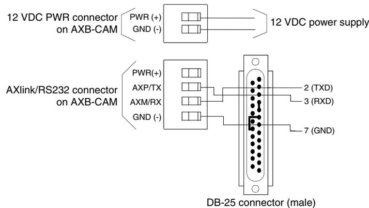
FIG. 9 AXlink/RS-232, DB-25, and power supply wiring diagram
