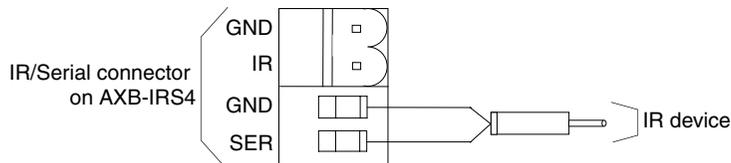
FIG. 11 Serial device wiring diagram
