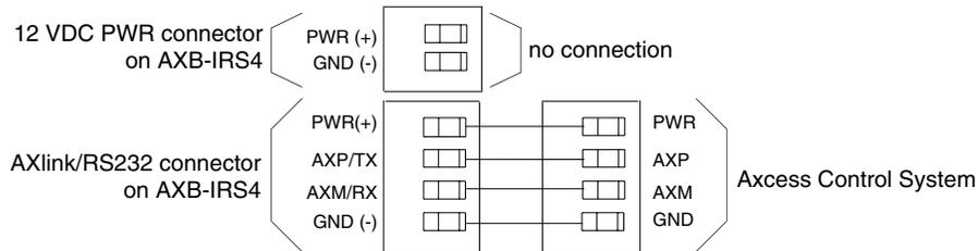
FIG. 6 AXlink data and power wiring diagram
