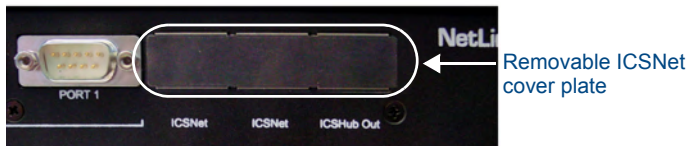
FIG. 2 Identifying upgradeable units (not ICSNet-ready)
