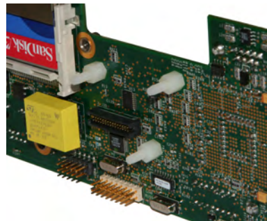
FIG. 4 Nylon hardware on motherboard
