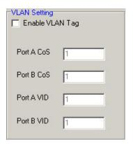
In **VALN Setting**, check the box of **Enable VLAN Tag** to enables to set up VLAN Tag as the four listed items.
