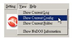
**Show Current Config** is to open a notepad for the current configuration file (\*.ini) of a loaded model to show its environment and detailed parameters of each task.
