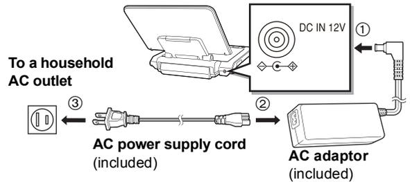
The unit is in the standby condition (the [⏻] indicator lights) when the AC power supply cord is connected. The primary circuit is always "live" as long as the AC adaptor is connected to an electrical outlet.
