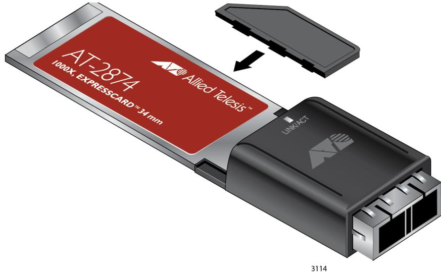
Figure 9. Attaching the Stabilizer to the AT-2874SX ExpressCard
