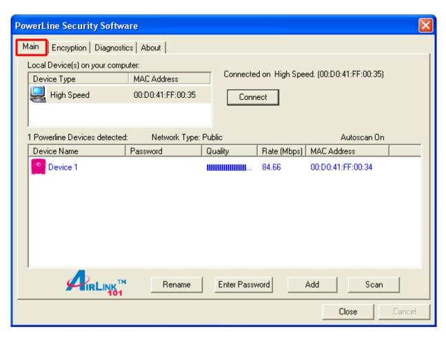
The Local Device is the powerline adapter connected directly to your computer. All other powerline adapters are listed under the Powerline Devices list.
